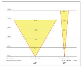
In lighting, choosing the lens angle is as important as selecting the color or wattage. Small angles retain brightness at long distances, while wide angles cover larger areas but lose brightness over distance.
